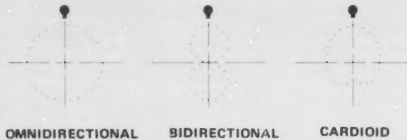
Illustration VII-7 Polar Patterns of Microphones
