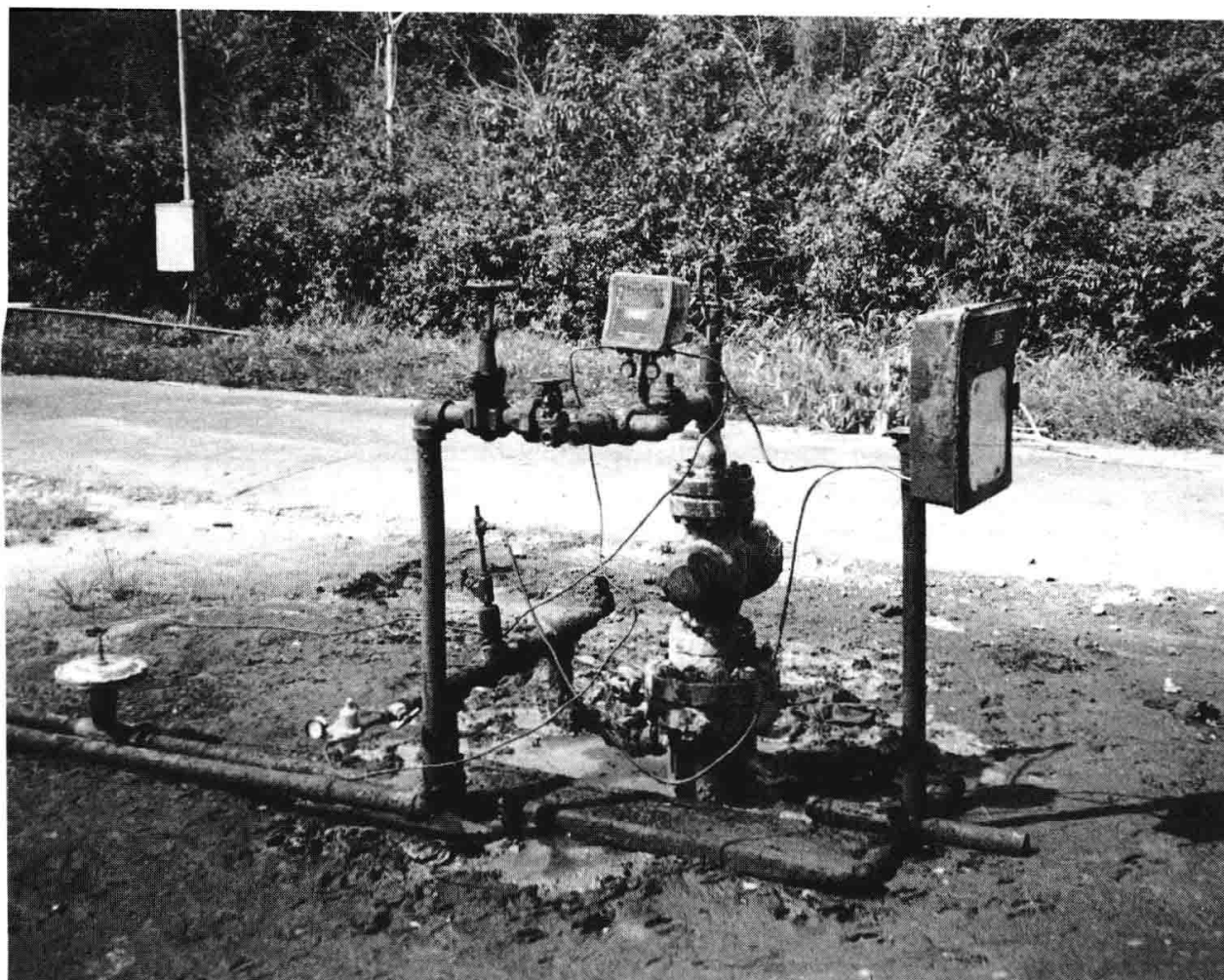
Figure 10.6 Injection equipment at the wellhead. There is not much to be seen: just the valving of the wellhead itself together with the water line, gate valves and gauges. This injection facility was actually being used for a microbial flood. ( Photographed in Oklahoma ).
