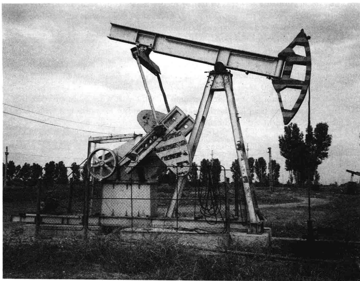
Figure 10.5 A typical wellhead pump. The oscillating boom, operated by an electric motor, actuates the pump via a string of rods extending to the bottom of the well. ( Photographed in Romania ).
