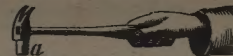
A MAGNETIC HAMMER. a represents the hammer attracting to it the tack b.
