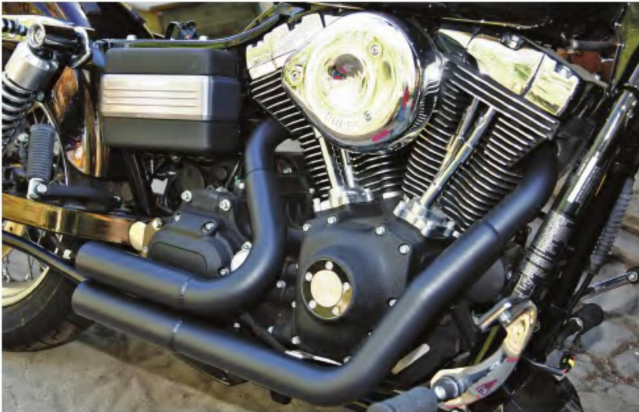
8. The new head pipes fit nice and close to the motor. Their black finish really matched the motor’s color. The sensor’s wires fit into the factory clamps.
