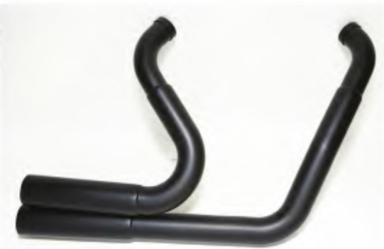
2. The head pipes have a three-step design, their flow capacity increases, so that the exhaust gas can expand as it moves down through the pipes. Their larger end fits onto the front of the muffler.
