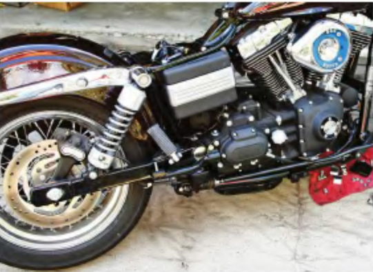
4. Once the electrical connectors were disconnected, removing the factory pipes was just like any other Harley. The stock muffler mounting bracket was also removed from the rear of the transmission.
