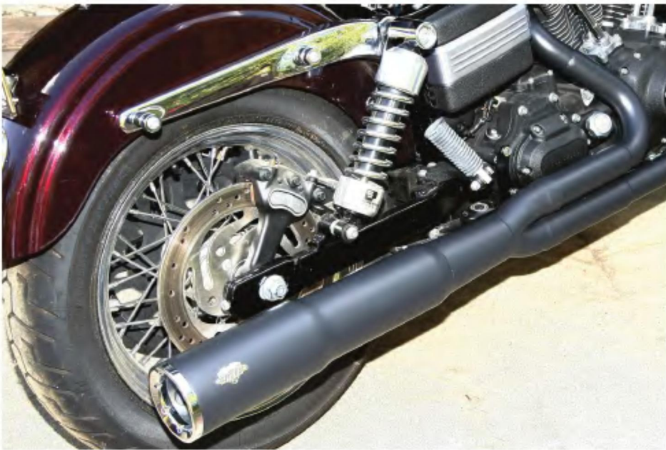
9. Installing the V-H muffler completed the mechanical part of the job, then it was time to fire the motor up and check out it’s sweet sound.
