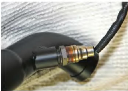
7. The oxygen sensors must be switched from the stock head pipes to the new pipes. Handle them carefully, they are expensive. Also rub a few drops of anti-seize on the sensor’s threads.
