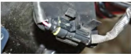
6. The connector for the front oxygen sensor is attached to a plastic plate that is sandwiched between the voltage regulator and the frame. You have to unscrew the voltage regulator to get to it. The connector for the rear oxygen sensor is in the wire harnesses under the seat. We found it by tugging on the wire down by the pipe and watching to see which connector moved in the cavity under the seat.
