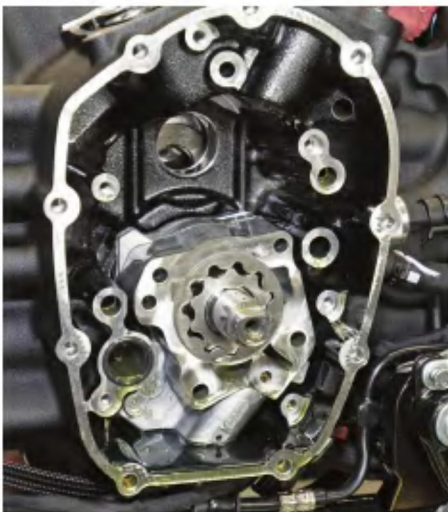
6. The Milwaukee-8's oiling system consists of a pair of gyrotor oil pumps, the pump housing, its back plate and a pressure relief valve. The pressure side of the oil pump (shown) uses a ten-lobe gyrotor pump that fits inside of the oil pump housing.
