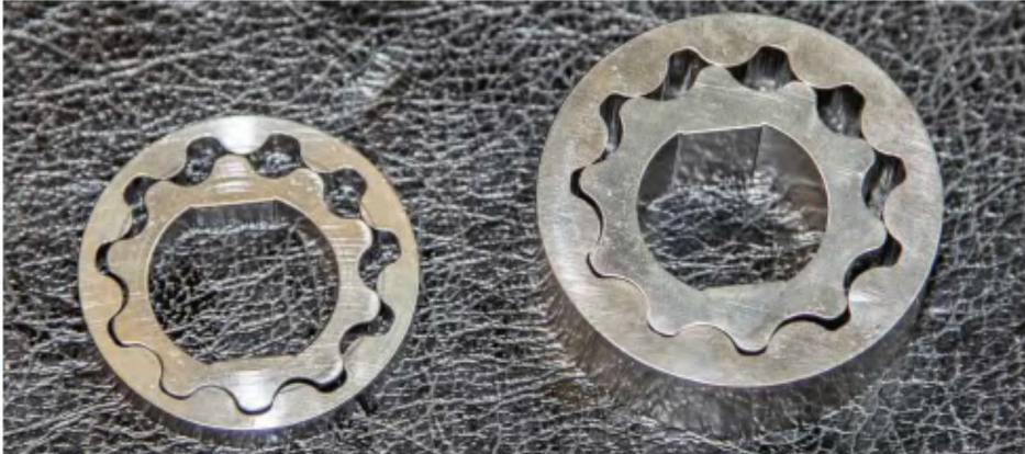
9. This is a comparison of the pressure side gyrotor assemblies of the Twin-Cam motor, left, and the Milwaukee-8 motor, right. The Milwaukee-8's larger gyrotor assembly should about double its oil volume to the motor's internal parts.
