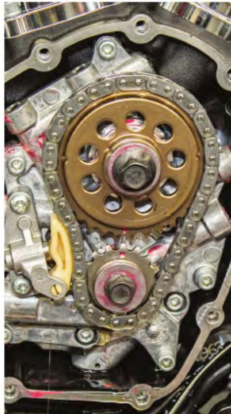
2. The layout of the parts inside has a similar appearance to the Twin Cam motor. The cam drive chain comes off as a unit with sprockets. Note the red timing marks on the sprockets, they must be aligned when installing the chain.
