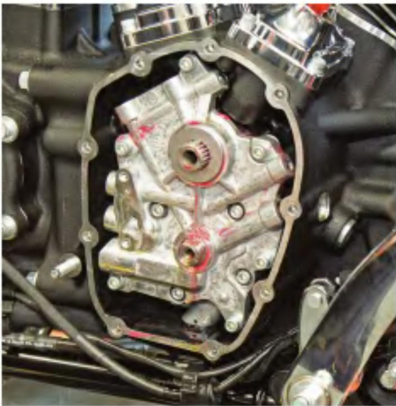
3. The cam plate is secured with six Allen head bolts and the oil pump is attached to the cam plate with four Allen head bolts. This cam plate is pressure die-cast. It features integral bearings for the crankshaft and camshaft. To pull the cam plate, you must remove all ten of these bolts. The oil pumps will stay mounted on the right end of the crankshaft.
