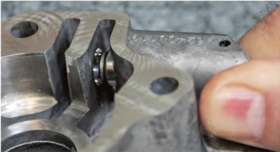
8. The pressure regulator piston seals against a port on the inside of the oil pump housing. The oil pressure regulator valve consists of a steel piston, which has a step on its head, a compression spring and a split pin that holds them inside of the cam plate.
