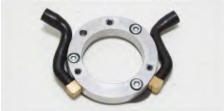
5. The air filter's breather system uses molded hoses and an adapter ring to connect the cylinder heads' breather ports to the inlet of the throttle body.
