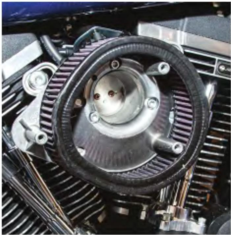
9. The washable filtering element fits tightly to the back plate assembly.
