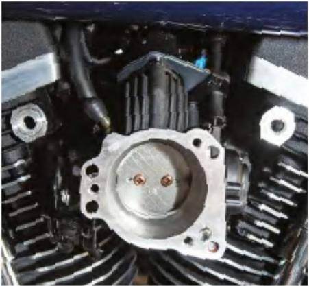
4. Our starting point: we have removed the stock air filter and its housing.
