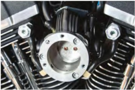
7. The breather's molded hoses are fitted to the air filter kit's banjo bolts, which are then fastened to the heads' breather ports.
