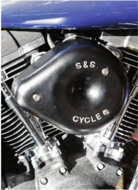
10. The outer cover was then secured to the back plate by three screws, on which we again used blue LockTite.
