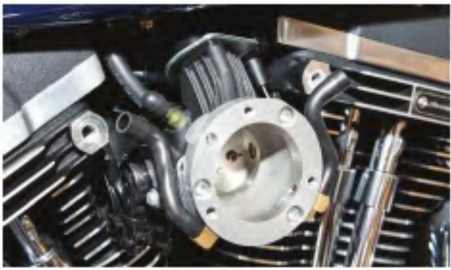
6. We have attached the aluminum breather adapter to the motor's throttle body.
