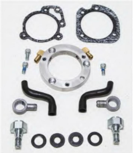
3. The other sub-assembly is the cylinder breather system; it feeds the motor's oiling system residue into the throttle body throat.
