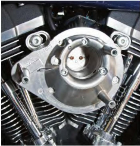
8. The air filter back plate is secured to the throttle body adapter with three screws; we used blue LockTite on the screws.
