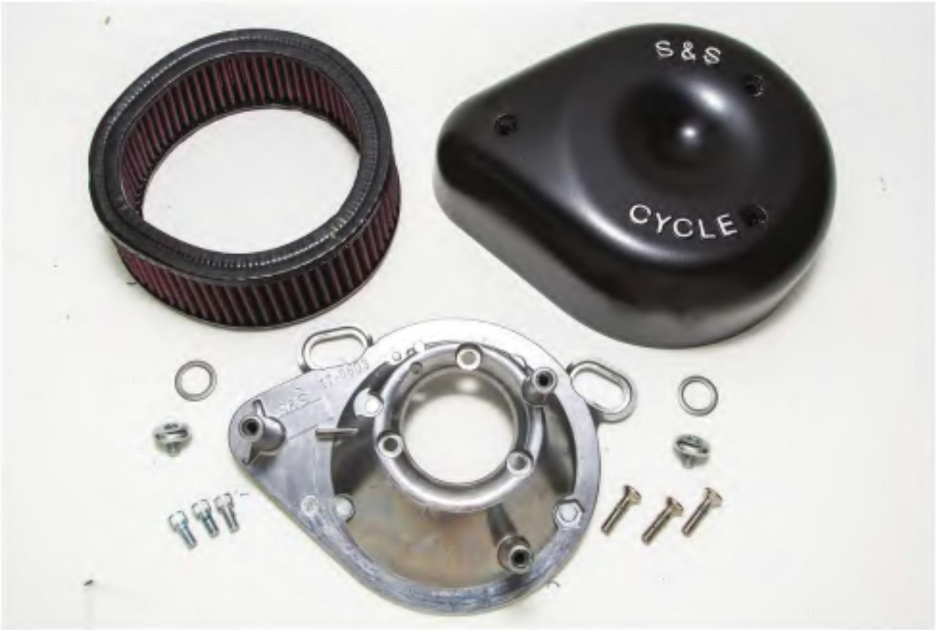
2. The kit's air filtering sub-assembly is made up from three main parts: the back plate, the filtering element, and the cover.
