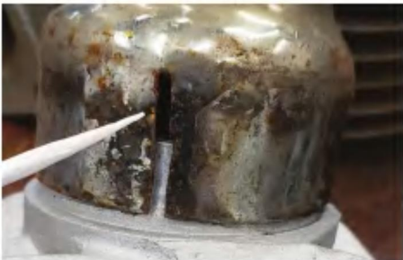
6. Just one of the many reasons our beloved Panheads can have exhaust leaks. The devils in the details.
