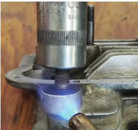
2. Always preheat the base material before removing the hardware.
