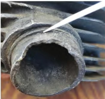
1. A chipped and very unhappy spigot. This one's gotta go!
