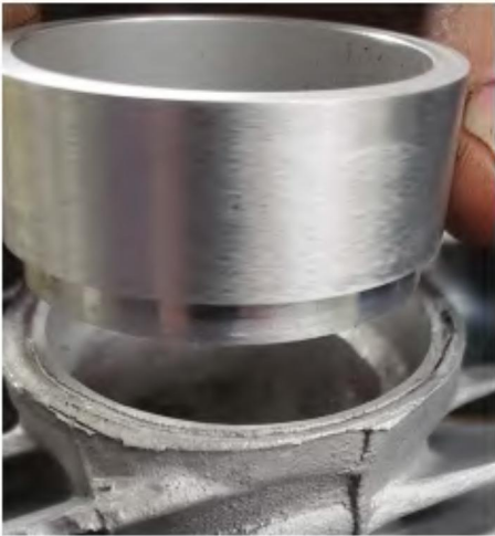
9. Perfect fit, time to weld on the inside.
