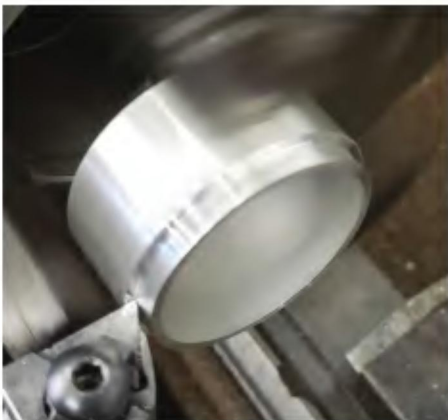
5. Machining the 6061 exhaust spigot. Notice the step that will receive into the bored head.
