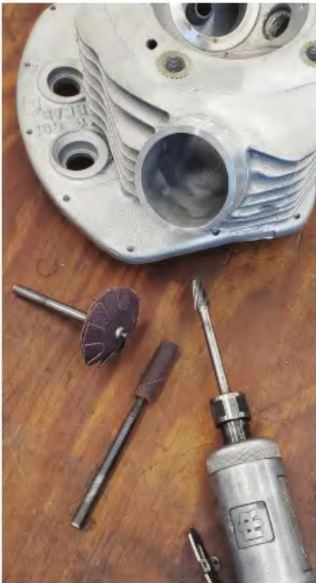
10. Tools for finishing the welded port spigot.
