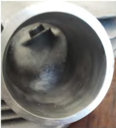
11. Finished exhaust port.
