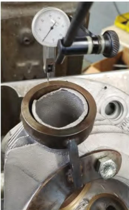
4. Indicating the fixture for finding level and zero prior to removing and boring the exhaust port.
