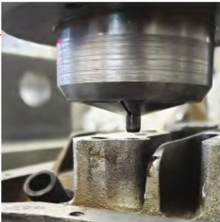
3. Preheated and now using the mill collet to remove the rocker bearing dowel.
