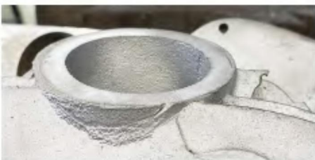
7. Exhaust spigot removed.
