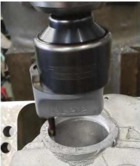
8. Boring the exhaust port to receive the new spigot.
