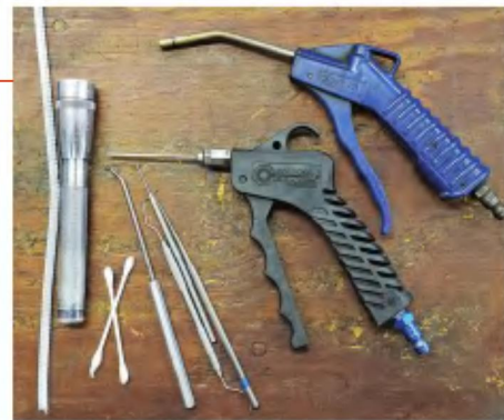
A sample of some of the instruments used in cleaning preparation. Of these, the needle blower and flashlight are most used. Needle blowers are a must.
