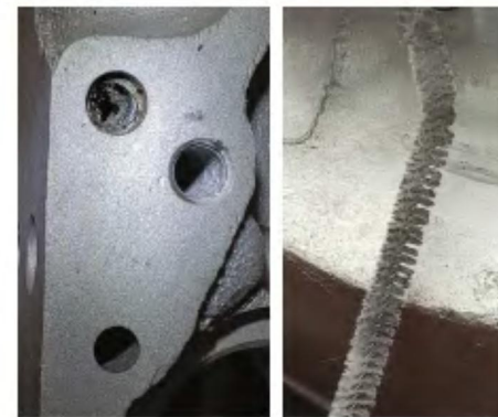
Oil passage area, after the lifter screen, showing old glassbead and other contaminants (top left); Dirty pipe cleaner from oil passage. This is from a very clean crankcase (top right).
