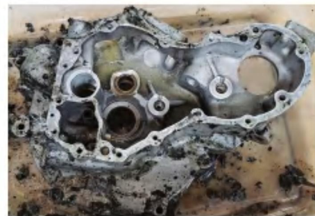
Stripping paint. It's better this way than to dirty up and waste glassbead.
