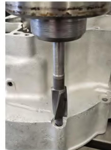
Cutting the hardware decks with piloted counterbore cutter
