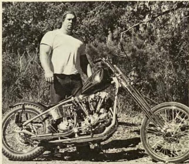
The curved brake pedal was moved back from the stock location and welded directly to the end of the cross-shaft. Note the chromed oil pump, lifter bases and cam cover.
