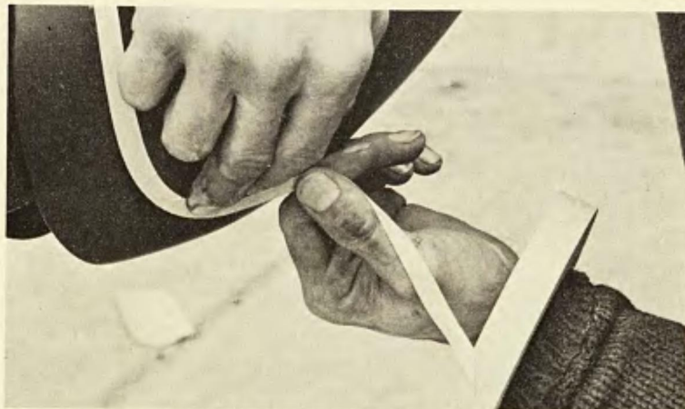
Start with \frac{1}{8} -inch tape, and try not to stretch it.
