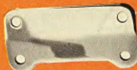
9108 Headlight Bracket. Used on FX and XLCH H-D when extended front end is used. Lowers headlight for easy adjustment. 4.50
