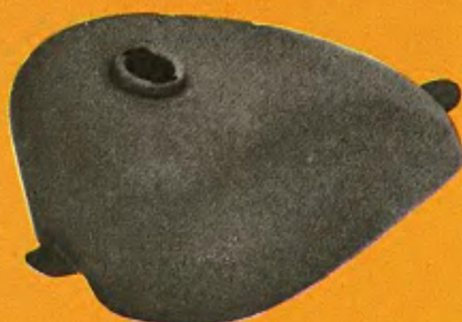
36024 Sportster Type Tank. Holds 2.5 gallons. Low tunnel. Made of steel. 39.95
