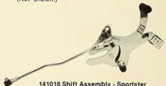
141016 Shift Assembly - Sportster '54 - '74. All Linkage included. Use Stock Shifter Peg. 79.25
