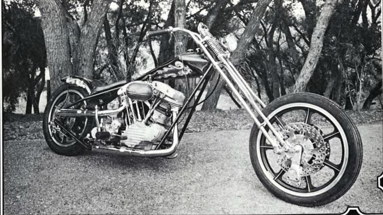
Fat Frank's Shovel: A 1947 lower end attached to a 1975 top end, balanced with lightening gears, Manley valves, and a late-model oil pump. Oil is stored in frame tubes and under gas tank. Tranny 1950 with Andrews 1st and 3rd gears, front dual disc brakes and rear disc, front 19-inch Morris Mag and rear 18-inch Morris Mag. Brake controls, chainguard, license plate mount, and pipes handmade and everything attached with countersunk allen bolts.
