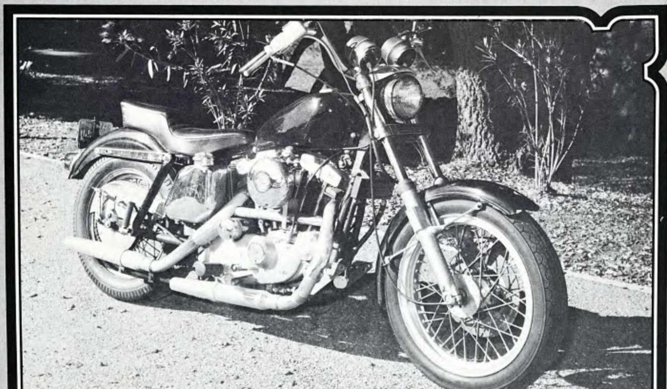
Tex's Sporty: 1976 XL-1000. 16-inch rear wheel, custom hand-rubbed lacquer paint. Stock shocks removed, rear end lowered 1 3/4 inches. Custom struts by Bandit. Stock air cleaner replaced, oil tank, chainguard chromed. Stock turn signals modified. Texas exhaust system with early Sportster mufflers.
