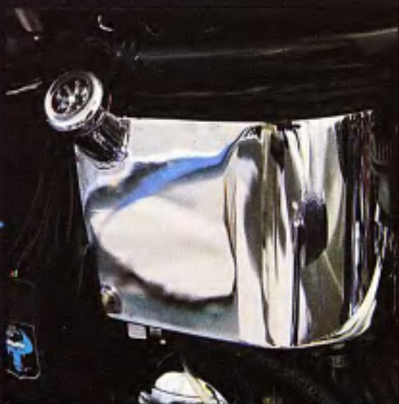
Custom chrome oil tanks with temperature gauges.
