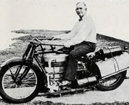
Builder is shown on steam motorcycle which operates smoothly at all speeds. A faint chug when it starts is the only noise
