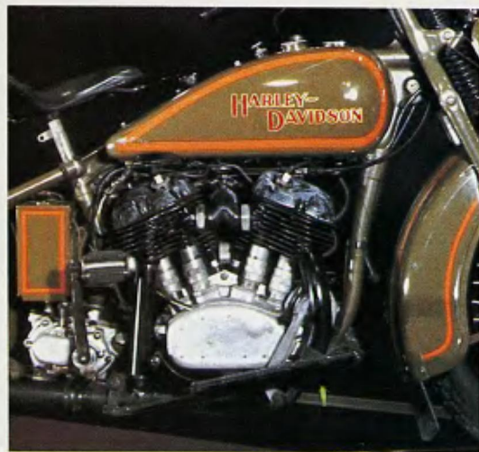
A high compression side-valve engine and olive drab paint made this second generation 74-inch VL model quite popular.
