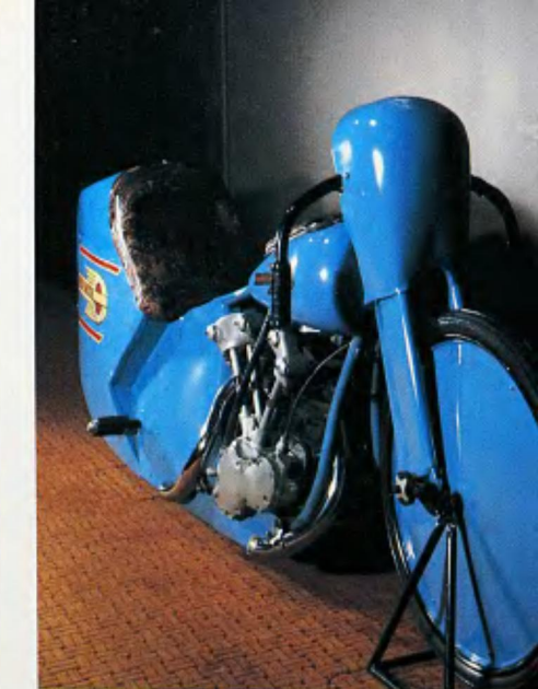
To promote the new OHV 61-inch series, H-D produced an alcohol-fueled, twin carb version that turned 136.183 mph.
