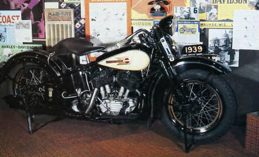
Most powerful of its time for sidecar usage, the 80-inch ULH V-Twin is a highly prized item for collectors.
