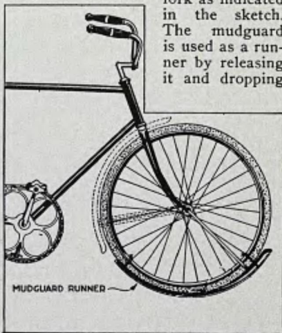
The Mudguard is Fastened to the Rim of the Wheel and Acts as a Runner over Ice and Snow
