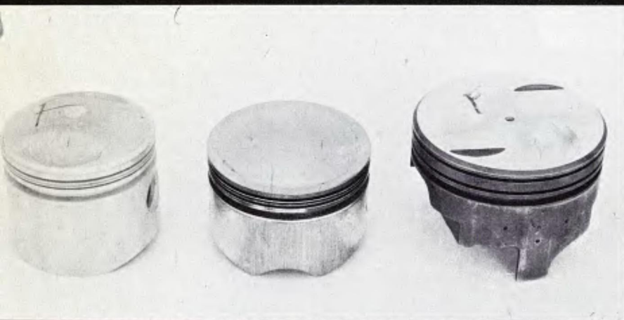
Pistons (left to right): stock H-D, S & S, 454 Chevrolet
