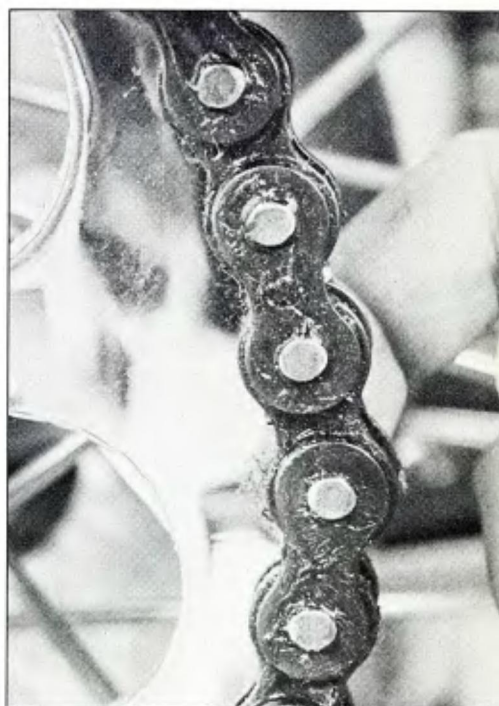
This sprocket was cut wrong an' it's gonna take the chain out in a few thousand miles. Sorry, bro, but there ain't very many good chain wheels bein' made these days, includin' the factory's — which this one is.
