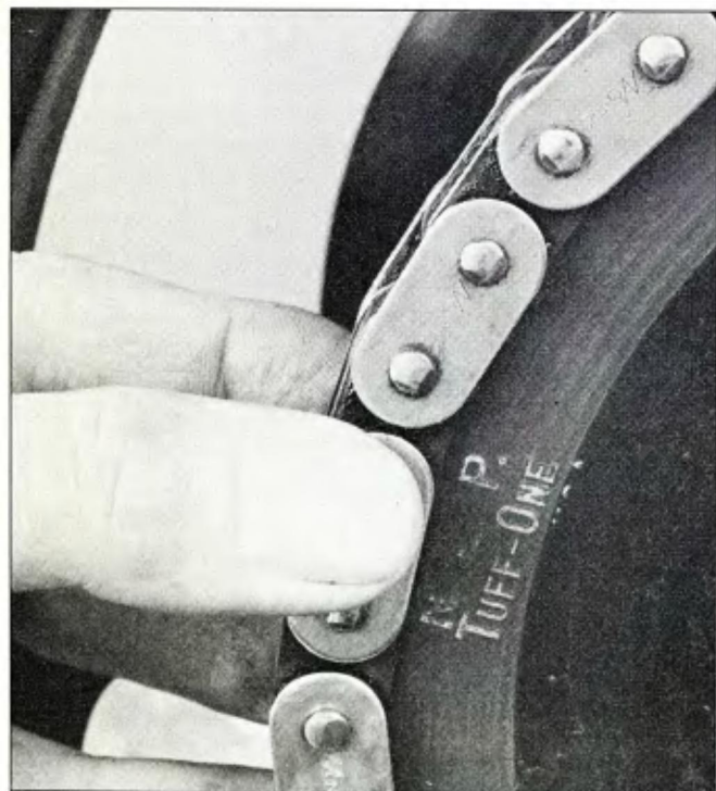
When the sprocket's cut right an' the chain is new, ya won't be able to pull the chain away more'n a quarter of a tooth. A new chain on a bad chain wheel is a waste of money.
