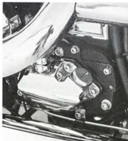
Oil pump painted to match engine
