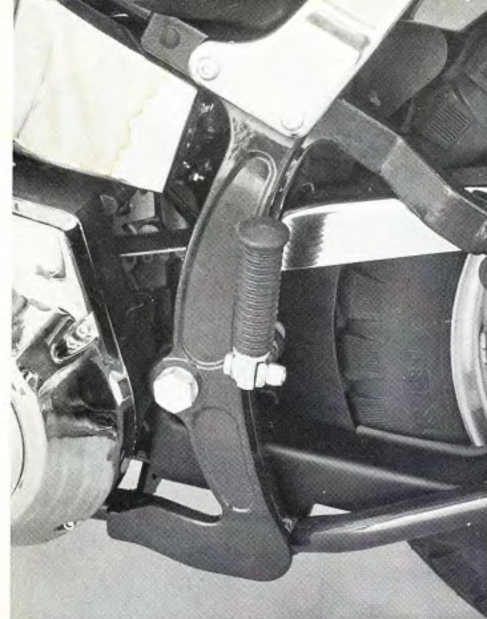
Heavy-duty casting adds rigidity
