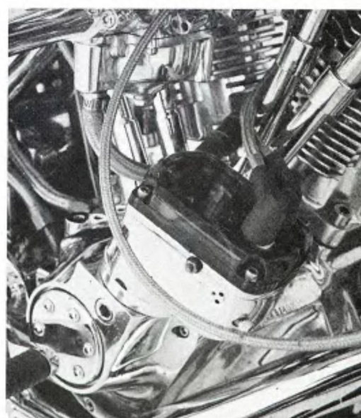
Magneto keeps fire burning
