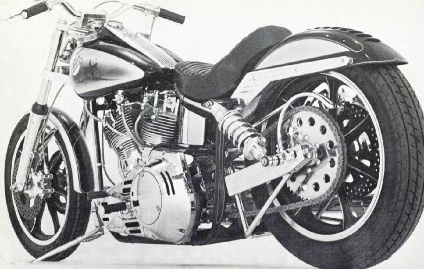
Double-thick swingarm is built to take anything the road can dish out
