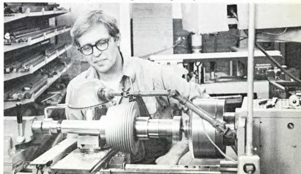
An XR750 cylinder gets metal removed from its base to adjust the compression ratio to about 12.75 to one. The cylinder-holding fixture is rigid and precise — a work of art.
