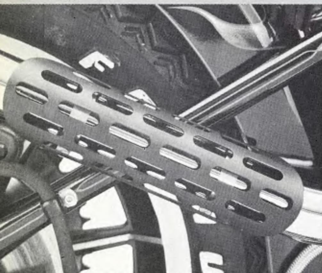
The heat shield — hot it's not, thanks to slots
