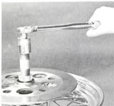
Axle nut must be torqued correctly when measuring end play.
