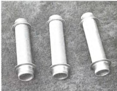
H-D makes wheel bearing spacers in three lengths. One of them should make things right.
