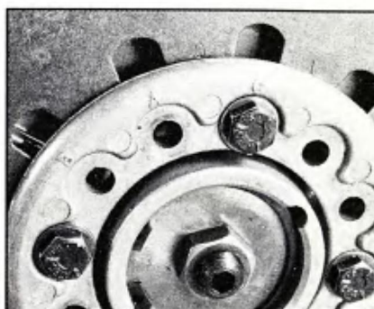
Harley's Evolution clutch is sure different from the traditional one. It'll handle more torque, but not more heat. The left photo shows all the parts of the new clutch. Center is a shot of the assembly; notice the automotive-style diaphragm spring. The aluminum collar that compresses the spring (right photo) also adjusts the spring shape, which is critical for best clutch feel and performance.
