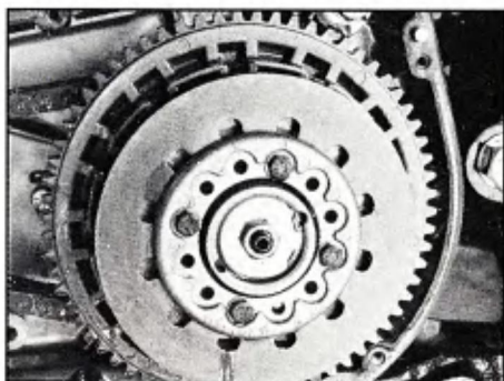
Harley's Evolution clutch is sure different from the traditional one. It'll handle more torque, but not more heat. The left photo shows all the parts of the new clutch. Center is a shot of the assembly; notice the automotive-style diaphragm spring. The aluminum collar that compresses the spring (right photo) also adjusts the spring shape, which is critical for best clutch feel and performance.
