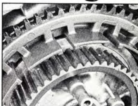
Clutch spring shape can be measured with ordinary tools. Note that the four spring retaining bolts are fitted through holes with a letter — either A, B, or C. These hole sets pre-load the spring different amounts, changing its shape. Best lever feel results when the spring is flat or slightly dished (left photo). The large contact area of the new clutch hub eliminates wear and the sticking between the plates and hub.
