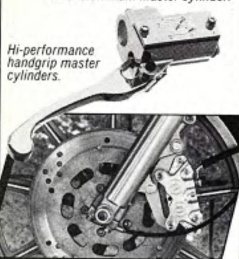
4 piston, 2 pad, dual action caliper for front/rear '84 & later FX, FXST & Sportster.
