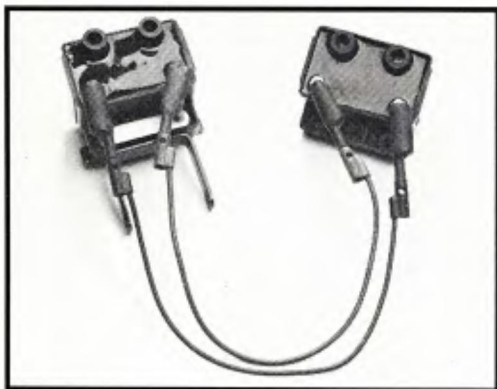
Photo #2: stock coils wired in series.
