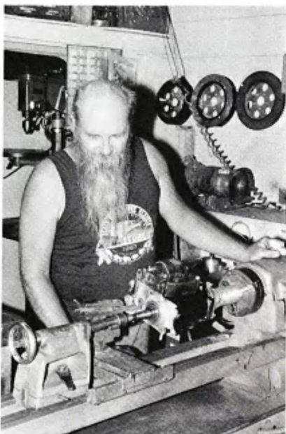
Phil Ross is a pioneer of belt-drive technology on Harleys. Here he demonstrates an easy way to turn down a tranny bearing boss without disassembling the transmission.
