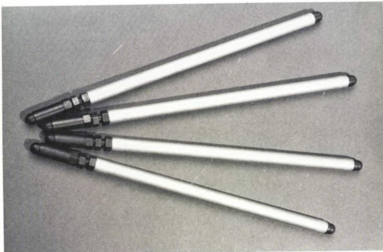
Adjustable pushrods will make top-end reassembly a helluva lot easier.
