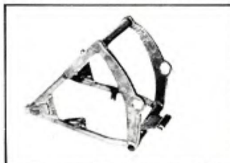
"BOLT ON" Adjustable Rear Fork Brace Raises and Lowers Rear with a Wrench
