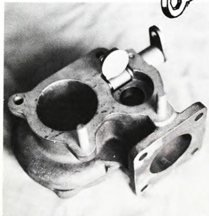
View of the built-in wastegate.
