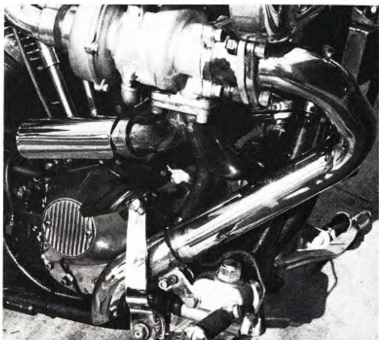
Exhaust manifold and refabricated pipe.
