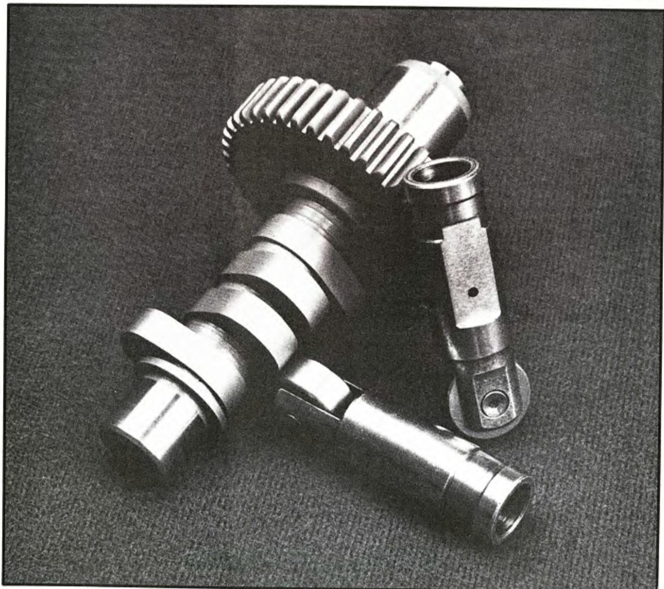
For good, lasting performance the Andrews "J" or "A" grind cams work well with standard hydraulic tappets.
