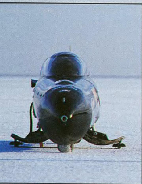
A small frontal area is the name of the game at the salt flat (stabilizer skids are retracted at speed).
