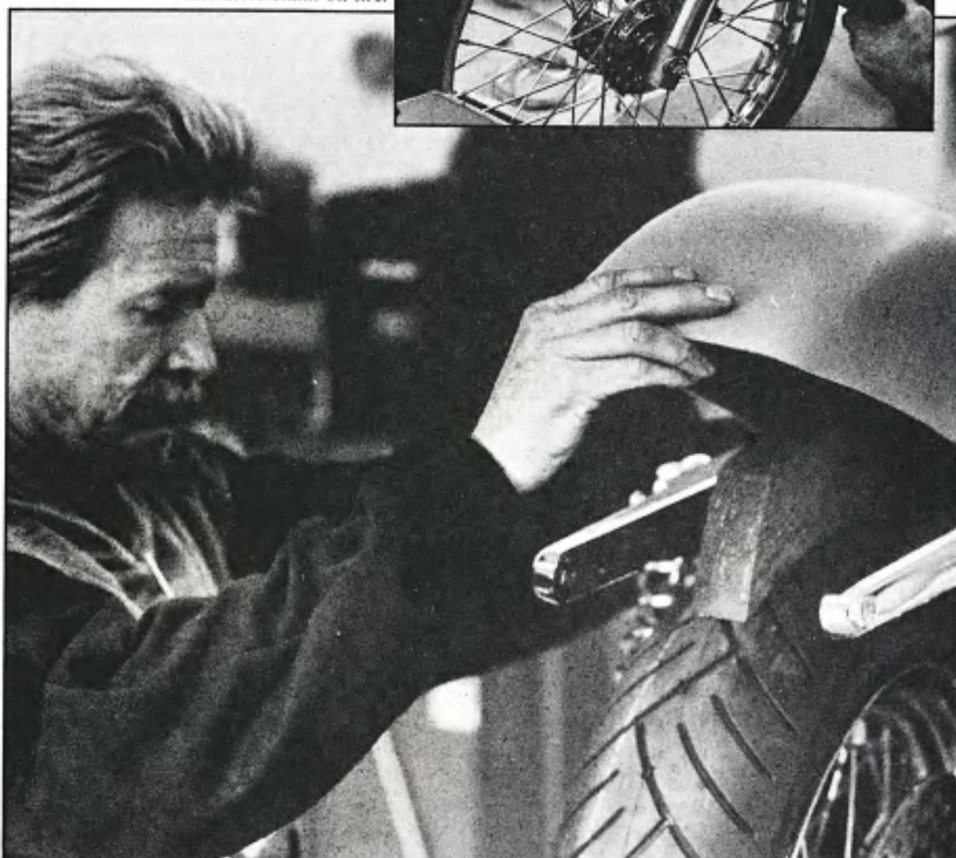
Arlen positioning fender on wood guide.
