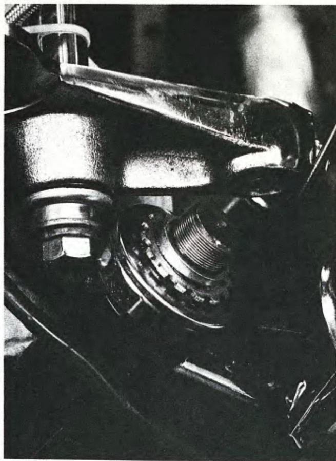
This is the special nut used to adjust the neck bearings. Check adjustment again after the entire front end is assembled.
