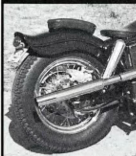
THE STRUTLESS® BIG-TWIN FENDER For Big Twins with four-speed frames. Fender will carry passenger's weight easily. All steel, mig welded. Requires very little molding, easily bolted on. Part #1010. Price: $159, shipping $10. U.S. Pat. #301391020. Bike pictured has short shocks #2222. Taillight: $19.95
