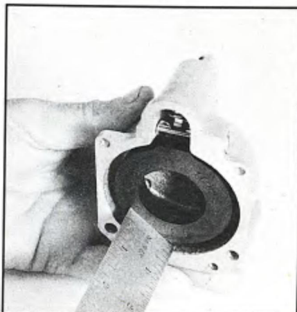
Photo B: Float bowl adjustment
