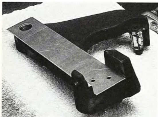
This shot shows Arlen's template in place. The tabs on either side need to be cut off with a hacksaw, then the holes must be drilled and tapped.
