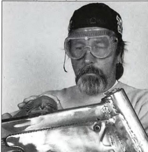
Finished grinding. Note the fork stop hole that's been drilled and tapped for the springer.
