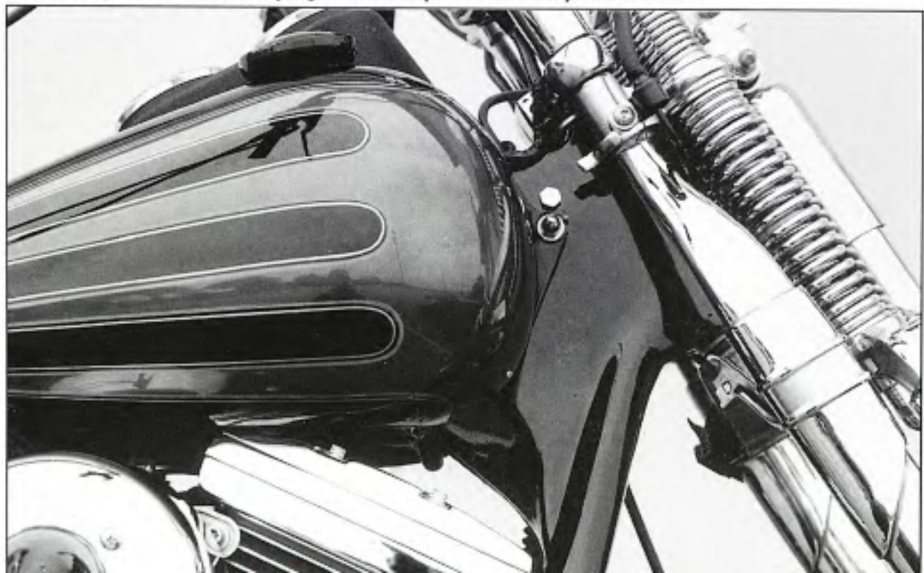
The completed neck with the springer and tank replaced. Not a bad job for a Hamster.
