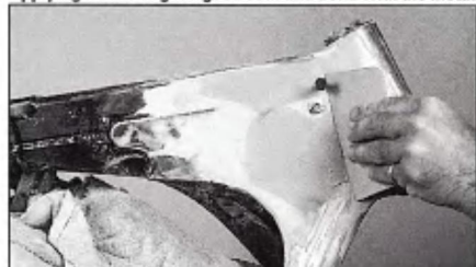
Bondo work complete and coats of primer being applied to allow inspection of work.
