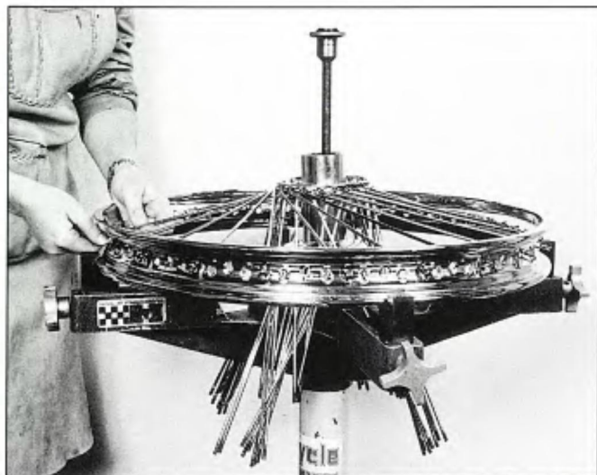
With the wheel and hub mounted on the Lacemaster, Brook starts the lacing process. This is a lot easier than working on the floor or a bench top.
