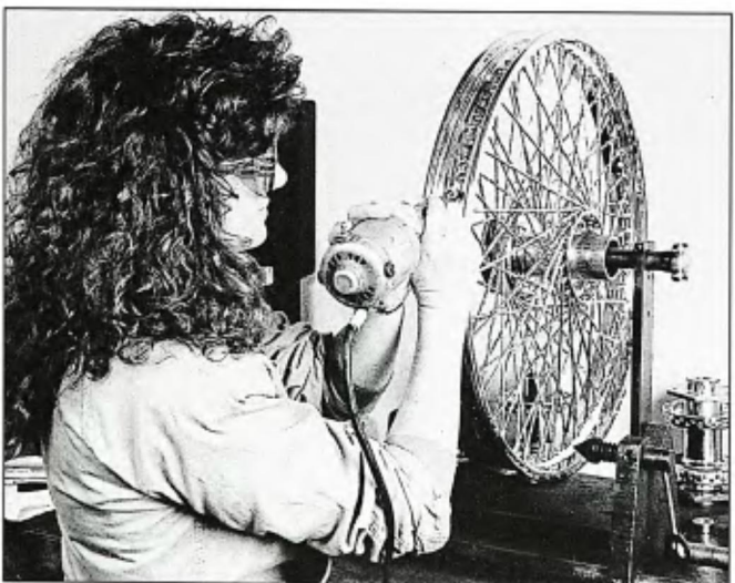
Threads protruding through the nipple are likely to puncture an innertube so she grinds off any excess and uses Loctite to make sure the spokes stay tight.
