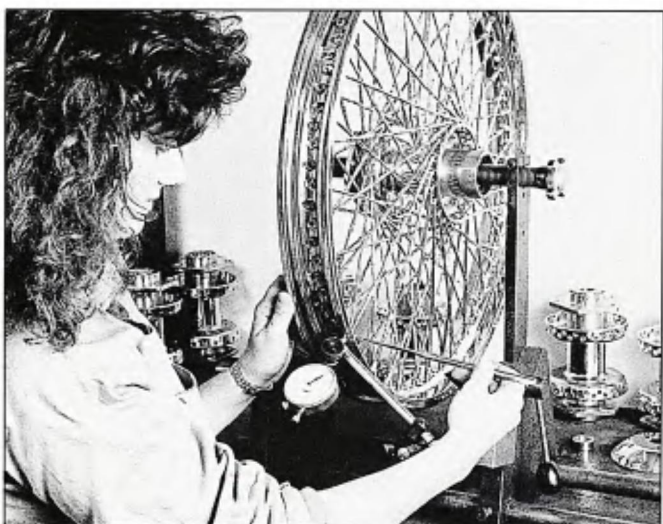
Brook trues the wheel up and down and side to side. With 80 spokes, this takes patience.
