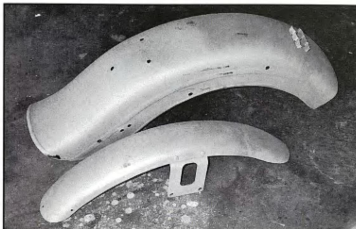
It is imperative that everything to be painted be cleaned right down to bare metal. Basic bodywork techniques fixed the fenders.
