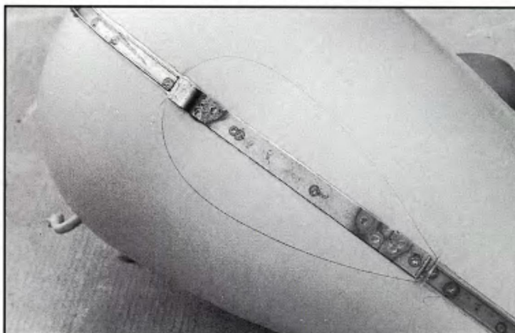
'46 knucklehead tank trim required attachment strips spot-welded to the tanks. Primer was ground for good electrical contact.
