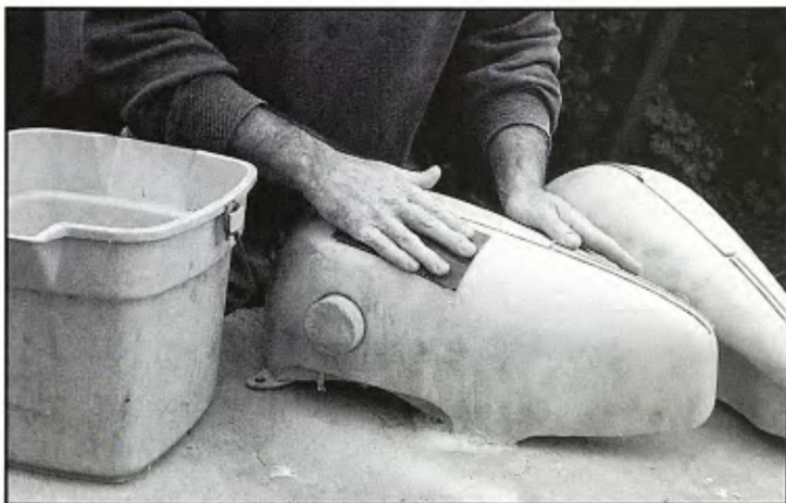
Primer builds thickness and block-sands (with 500-grit wet and dry) easily. Palmolive dish soap prevents fingerprints and clogging.
