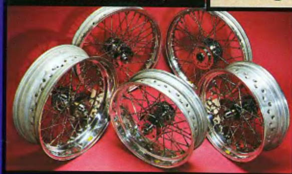
WHEEL ASSEMBLIES WITH WIDE AKRONT POLISHED ALUMINUM RIMS
