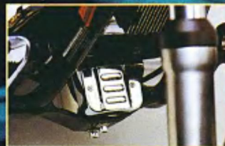
Chrome Lower Motor Mount Cover for Dyna Glide® Models Deeply stamped, "louer" styled chrome-plated top cover. Installs in minutes and is secured with chrome-plated countersunk screws.
