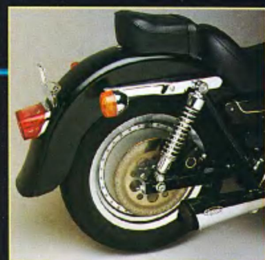
Heritage-Style Rear Fenders for FXR Models CCI's exclusive, all-new, steel fender lets you combine the Classic styling in an all-new, steel fender that mounts between the stock fender struts of all FXR models from 1982 to present.
