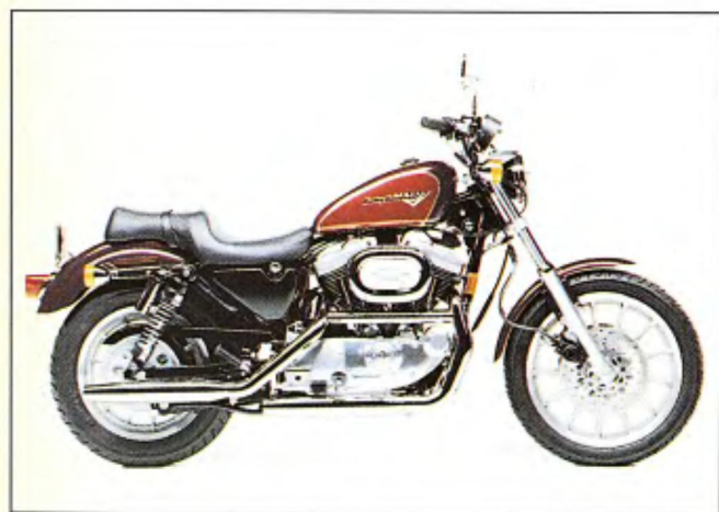
XL1200S Sportster Sport ($7,910 solid, $8,060 candy and $8,285 two-tone): The other new '96, this model carries the most sophisticated suspension ever put on a stock Harley. Both the cartridge-style fork and reservoir shocks offer adjustments for spring preload, compression and rebound damping.
