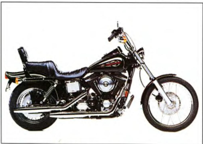
Dyna Wide Glide ($14,030 solid, $14,230 candy, $14,555 two-tone): The most custom Dyna, the Wide Glide offers a 21-inch front wheel, wide fork, flamed fatbob tank, forward-mounted controls and high bars. Battery box and electrical boxes have been restyled. For Dynas, add $285 for California models.
