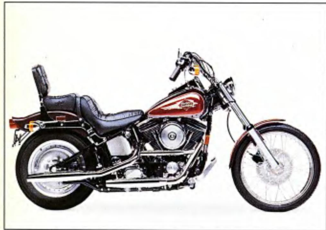
Softail Custom ($13,360 solid, $13,830 candy, $14,155 two-tone): All six Softails are powered by the 80-inch V-twin engine, and are solid-mounted. This custom has a 21-inch laced front wheel, 16-inch rear disc wheel, wide fork, and buckhorn bar.
