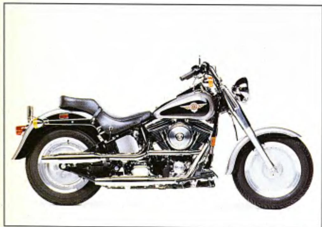
Fat Boy ($13,930 solid, $14,130 candy, $14,455 two-tone): Solid disc wheels front and rear, custom metal fenders, shotgun-style dual exhausts, floorboards, and a wide bar give the Fat Boy lots of class. All 80-inch Harley engines come with the five-speed transmission and belt drive.
