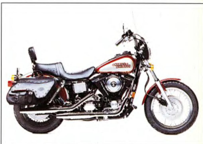
Dyna Convertible ($13,330 solid, $13,530 candy, $13,885 two-tone): The 80-inch V-twin engines on Dynas are rubber mounted so they don't shake much. This model "converts" to a custom when you remove the windshield and bags. Also has twin front discs and 28-degree sport chassis.
