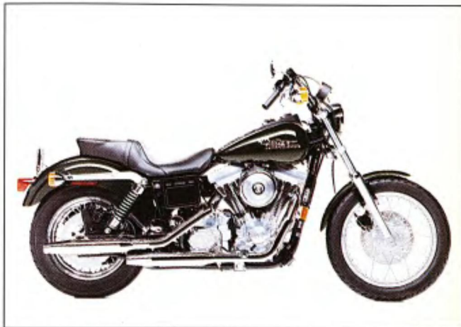
Dyna Super Glide ($10,195 candy, $10,345 two-tone): Dynas get a new frame that offers an .88-inch lower seat height. The least expensive Big Twin, the Super Glide has a dual seat, buckhorn bars, and black headlight bucket. Its narrow forks and 28-degree sport chassis give it a sportier ride.
