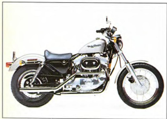
XL Sportster 883 ($5,095 solid, $5,245 candy): This solo-seat model is the least expensive new Harley-Davidson. It's powered by an 883cc, air-cooled V-twin engine and comes standard with a low handlebar and cast-aluminum wheels.
