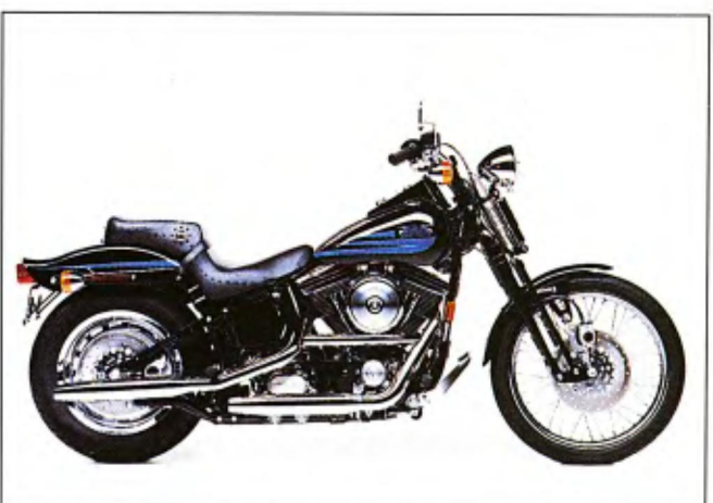
Bad Boy ($14,425 solid): The Bad Boy has the looks of a Springer, but features black forks, slotted disc rear wheel, and cloisonné tank emblems. The Bad Boy's sleek, blacked-out bravado is backed up by high-contact-ratio transmission gears.
