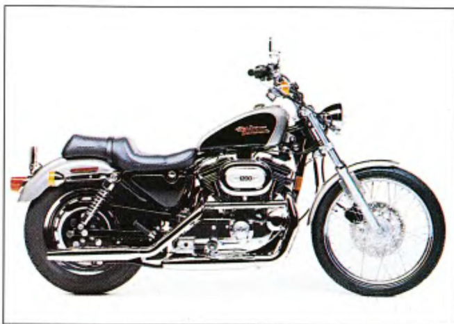
XL1200C Sportster Custom ($8,360 solid, $8,510 candy, $8,735 two-tone): One of two new models, it features a 21-inch laced front wheel, chrome stand-alone headlight, and handlebar riser assembly. Check out the chrome-and-black engine, low-rise handlebar, and custom slotted disc rear wheel.
