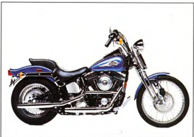
Springer Softail ($14,030 solid, $14,230 candy, $14,555 two-tone): Softails have a hard-tail look, but are suspended by a pair of shocks laid under the engine. With its exposed fork springs, the Springer looks like a '40s-era bike. The floating front fender moves with the tire.
