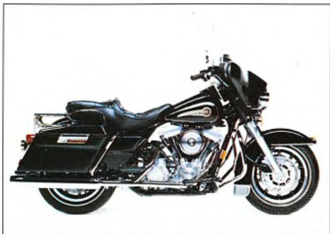
Electra Glide Standard ($12,235 solid; add $265 for Calif. models): The cheapest bagger, it has a fork-mounted fairing, saddlebags, and luggage rack. The inner fairing of the three Electra Glides has been redesigned for improved appearance and function. FLs use the 80-inch V-twin in rubber mounts.
