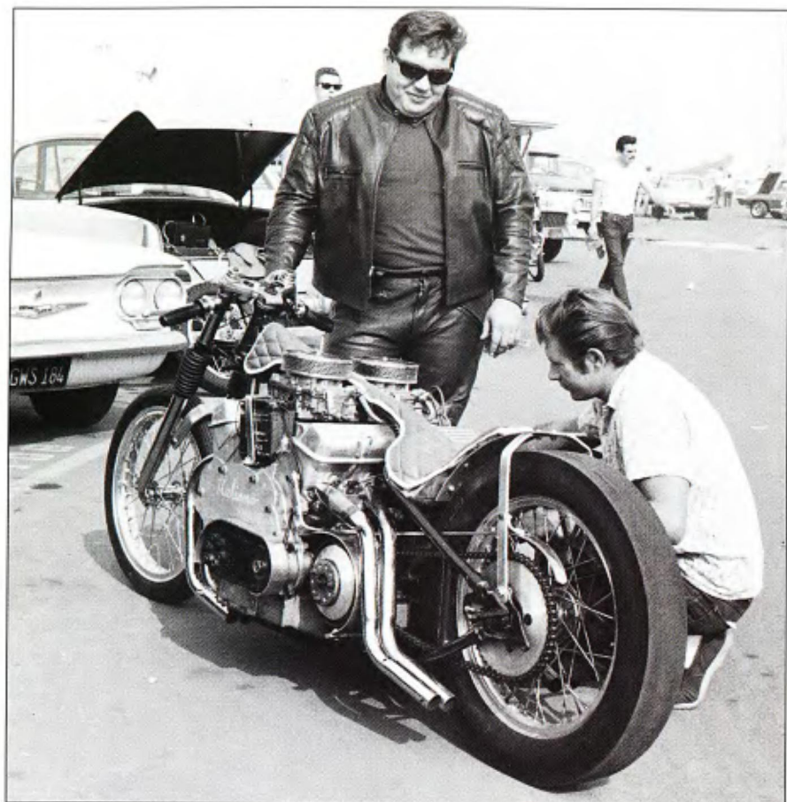
Joe (left) and Mil Blair (right) campaigned this Buick Aluminum V-8 drag bike in the mid '60s—capable of speeds of 160+ and low 9 E.T.s. It never realized its full potential due to the unavailability of a good "legal" motorcycle slick in the '60s.
