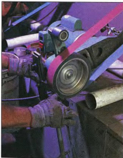
Belt grinding blade bevels
