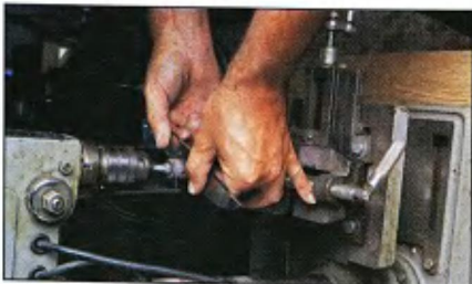
Grinding out finger release
