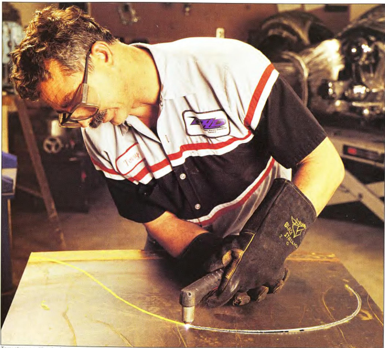
Terry plasma-cutting the fender panels.
