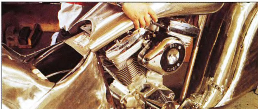
Stretched gas tank going into place.
