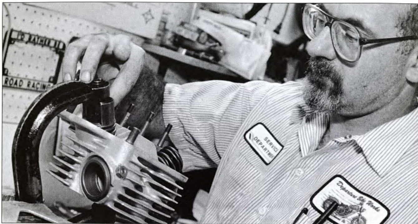
After checking for leaks, Musky installs the valves, springs, and keeper.
