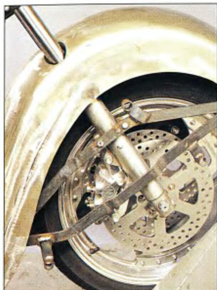
Front fender with panel removed.
