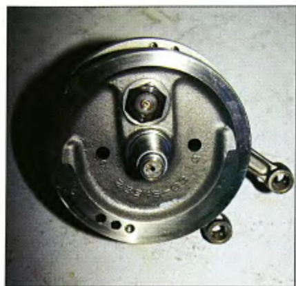
Broken pinion shaft.
