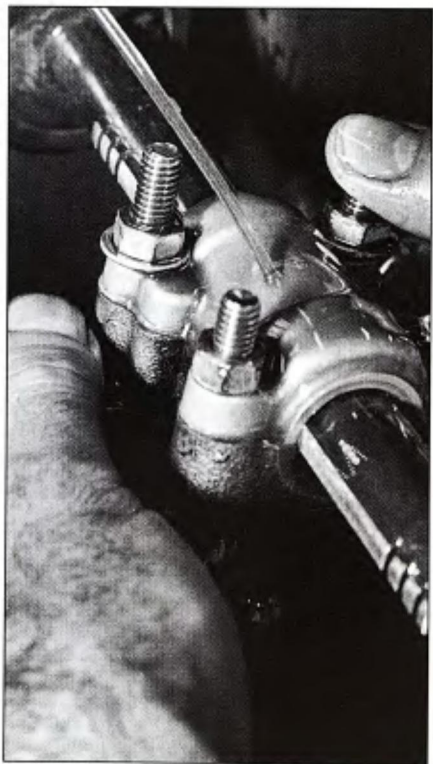
Honing a clamped set with a Sunnen Hone.
