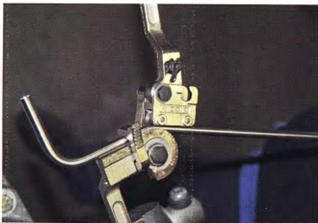
Mark's second bend is to position the tube next to the oil tank while keeping it behind the exhaust pipe. Knowing just where to bend the tubing and how much to bend it, comes from a lot of experience.
