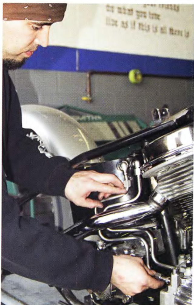
Once Mark has the tube finished, he fits both ends to each of their corresponding fittings before threading the flare nuts on. This way there is no stress or binding on the line.
