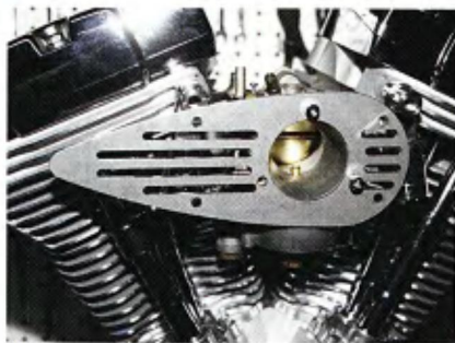
The back plate mounts directly the carb's air intake. This air cleaner is designed for use with separate cylinder head breathers.
