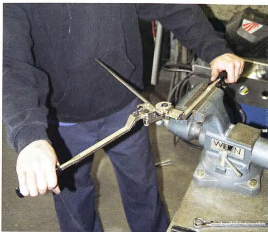
He uses a high-quality mandrel-type tube bender to keep from kinking the tubing.
