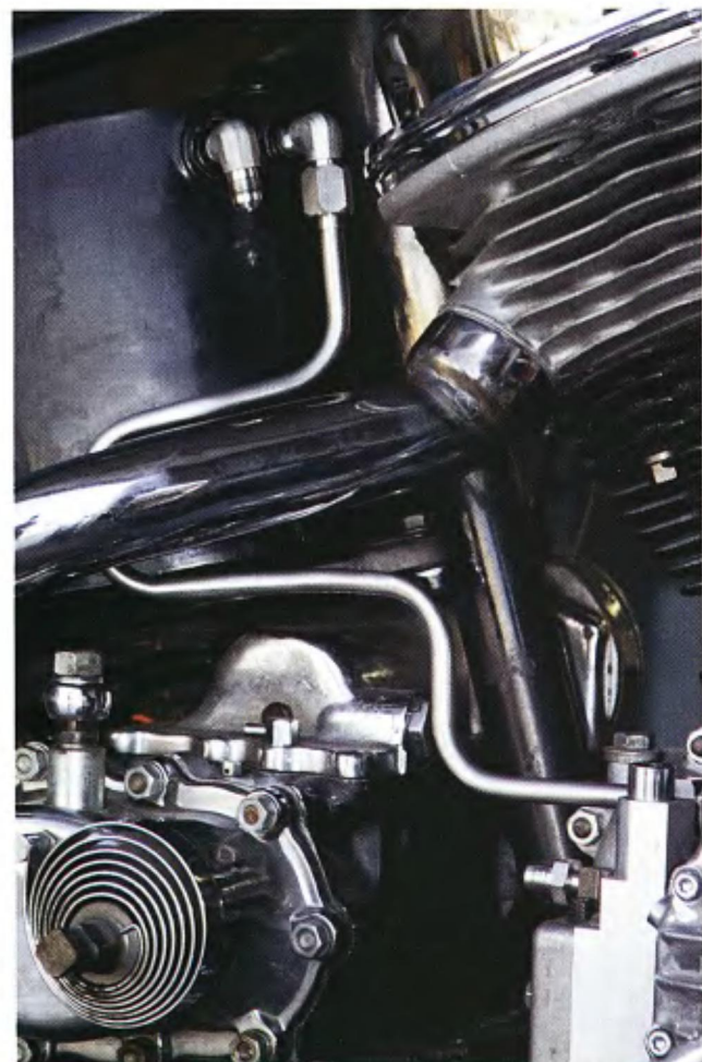
Mark's first step was to install aircraft-grade, 90-degree, -4 AN to 3/8 NPT elbow fittings in the oil tank and straight -4 AN to 3/8 NPT in the oil pump. The AN type of fitting uses a 37-degree flare; it is standard in the aircraft industry.
