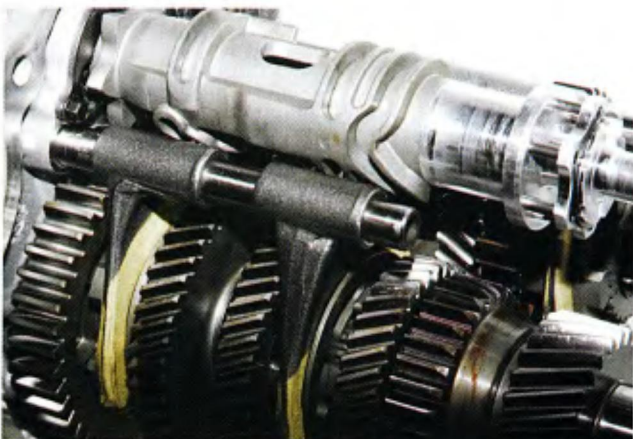
The 6-speed's shift drum is all new. It is hollow so that it doesn't have as much kinetic energy as a solid chunk of steel would have.
