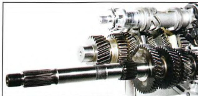
The one-piece mainshaft is a machined work of art. From the trap-door to the end of the clutch hub nut's threads, this one piece of steel. Last year's 5-speed used 20 parts to make this item.
