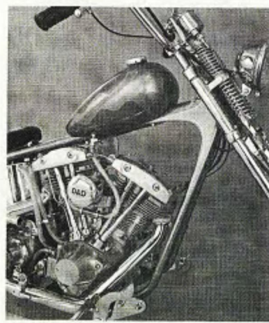
Long front tubes allow the use of a long fork without extreme neck angle or high center of gravity—this, along with solidly built and reinforced frame, makes the good handling and good looking combination possible.
