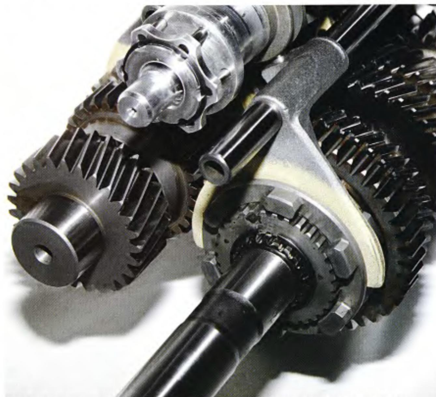
This is the business end of the three shafts that ride in those bearings. They are all highly polished, hardened steel.
