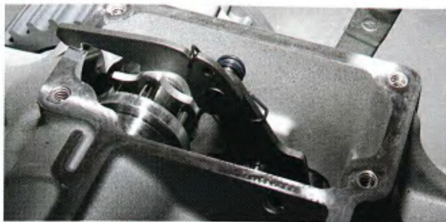
The shift arm is made from heat-treated steel.
