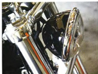
The stock headlight wouldn't look so out of place if Harley's new 49mm forks weren't so good looking. The triple trees are milled and polished aluminum forgings.
