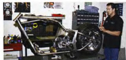
Mark sights down the string, so that it is centered over the frame's backbone.
