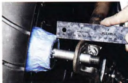
Because the spacers come in widths of 1/8-inch increments, a common ruler can be used to measure the distance. This spacer needs to be 2 inches wide.
