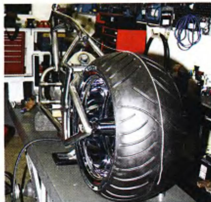
A length of string is tied to the steering head and draped over the rear of the bike.
