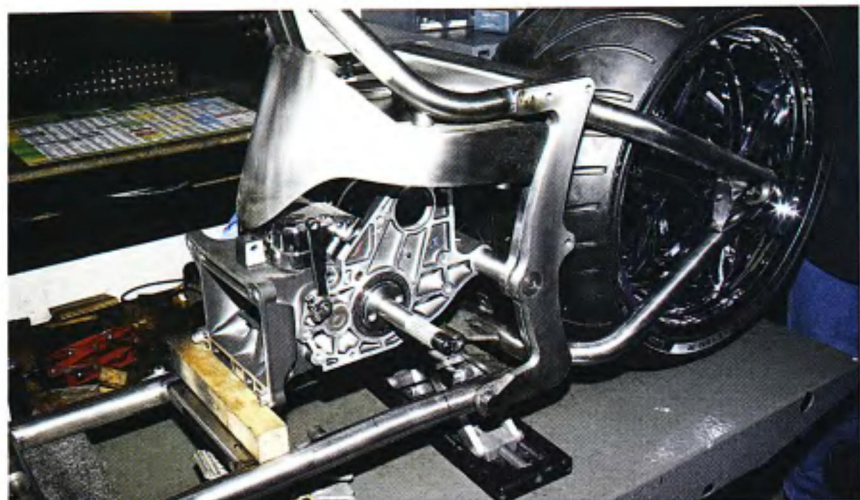
Mark has the frame and swingarm bolted together with a "B" series transmission attached to the swingarm pivot. The frame is jacked-up so that the rear tire is just off of the work table.
