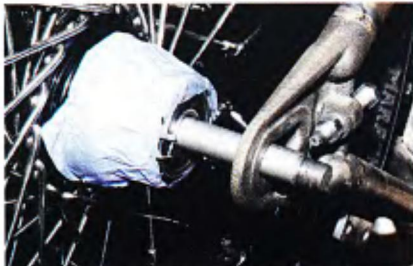
With the wheel centered, you get an idea of just how wide a spacer is needed in between the right side of the wheel and axle mount.
