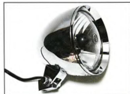
The stock headlight bulb assembly and wire harness fit into the Headwinds housing. Next, we installed the new headlight mount onto the headlight then bolted it to the bottom triple tree. The wiring was plugged back together, pushed back into the frame, and the grommet installed.
