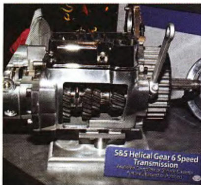
One of the great things to come out of this show were the cut-away displays. The new S&S transmission was killer, showing just how everything meshes together.
