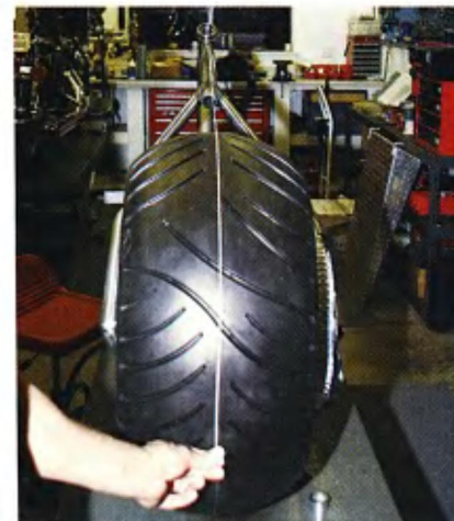
He has positioned the tire so that it is centered under the string. You can't get any better alignment than this.
