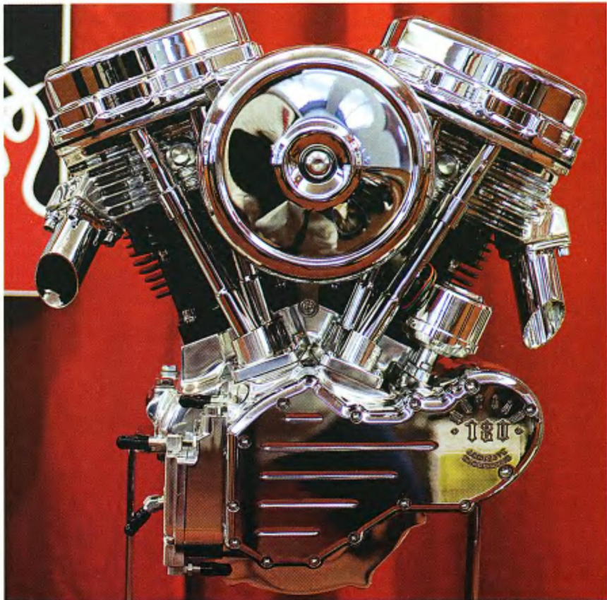
Here's the 120-cubic-inch panhead motor that garnered Accurate Engineering the award.
