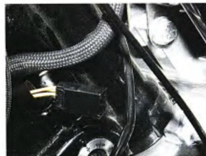
The connector for the headlight wiring is buried inside of the frame's fork neck. We removed the rubber grommet from the frame opening and then pulled the headlight wiring out until the connector was clear of the frame.
