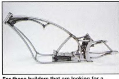
For those builders that are looking for a frame with rear suspension, Independent Cycle offers also the Lowlife frames that use a swingarm.
