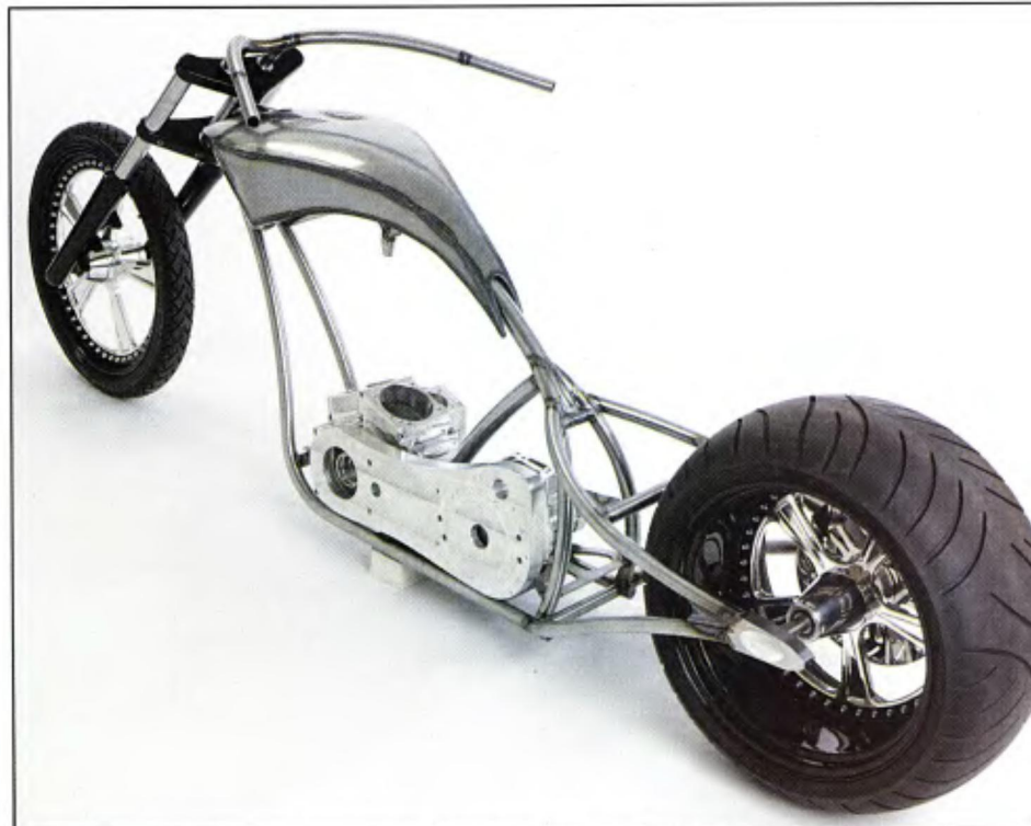
This rolling chassis gives an idea of just what can be done with the Hardlife frame. That's a 300mm rear tire on it.
