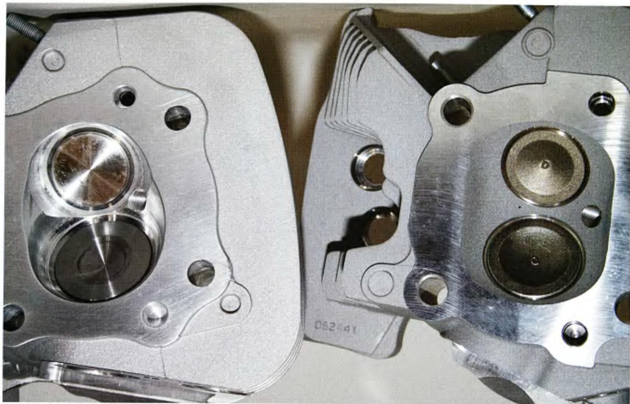
Here is our big deviation from Alan's Fatvo recipe; we used a set of S&S Super Stock performance cylinder heads (left), instead of stock Twin Cam heads. These heads use a 1.940-inch intake and a 1.575-inch exhaust valves. The S&S heads feature intake ports that are large enough to feed the 100-inch motor. The 79cc combustion chamber works out to 10.3:1 compression with the flat top pistons. If starting becomes a problem, the heads are machined for S & S electric compression releases.
