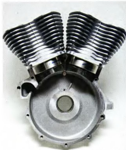
The first order of business is to trial fit the two cylinders on to the left side crankcase half.
