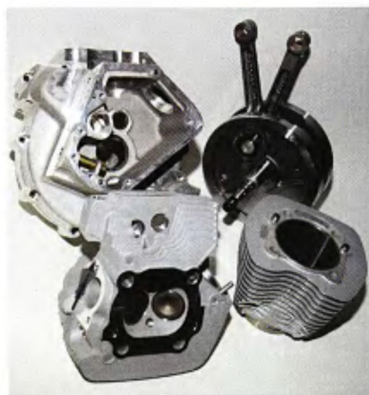
Here are the leading players in the building of a Fatvo motor: cylinder barrel and head from a Twin Cam motor, Evo flywheel assembly and the special cases from Sputhe Engineering.
