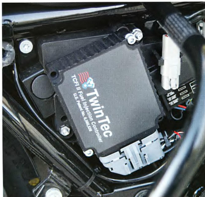
The Daytona Twin Tec ECM mounts in place of the stock fuel injection controller. It hooks directly into the factory wire harness. There are two modifications that are made to the harness for the oxygen sensor.
