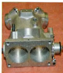
This is the Gerolamy dual runner throttle body that allows the fuel-injected motor to ingest enough air to take advantage of the hot cams and headwork. It can pass almost double the air of the stock single-runner throttle body.
