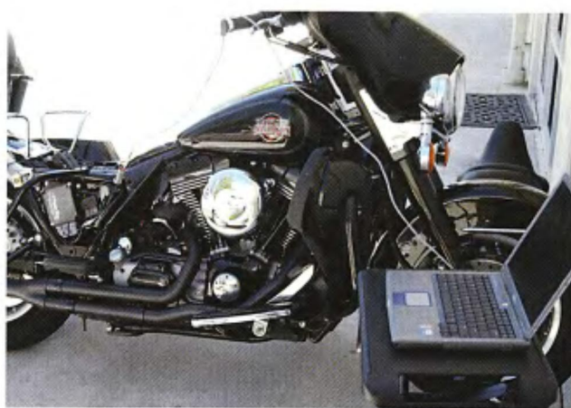
A laptop is connected to the ECM for basic setup. Once this is accomplished, the Daytona Twin Tec ECM relies on the oxygen sensor to keep the system adjusted for correct timing and air fuel operation.
