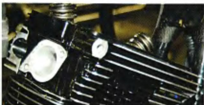
The B. C. Gerolamy reworked cylinder heads complemented the motor's breathing capacity. They now have 1.90-inch intake and 1.57-inch exhaust valves operating in CNC-matched ports.
