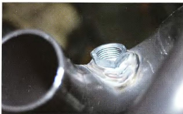
Bungs for the oxygen sensors were welded into each pipe.
