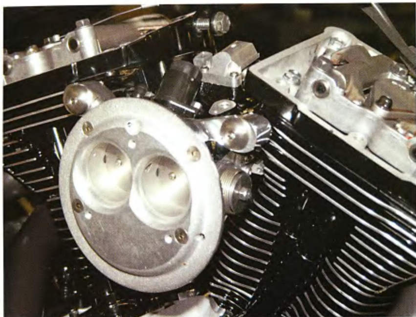
The dual-runner throttle body has a large diameter air filter back plate with blended air inlets for the two throttle bores. The back plate not only includes the cylinder head breather passages, but also acts as the outboard mount for the throttle body.
