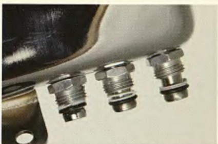
The other ends of the oil lines use compression fittings to attach them to the spigots on the oil tank. Each fitting has a compression nut, spiral type nylon washer and rubber O-ring.
