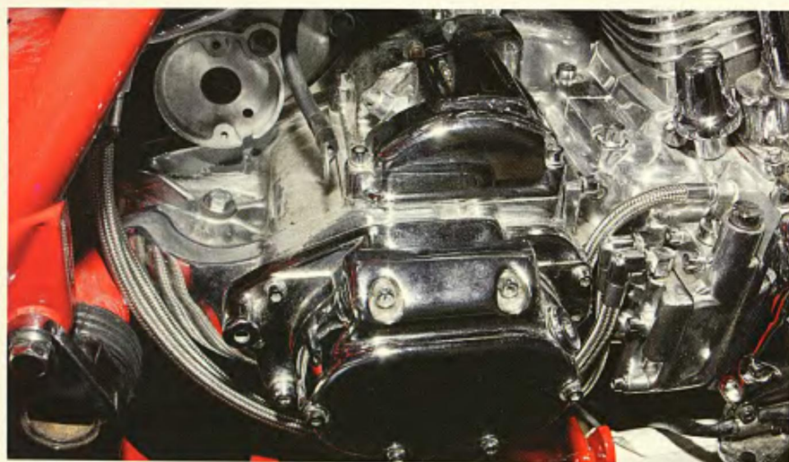
The right angle fittings on the ends of the oil lines just push on to the male fittings on the oil pump. This makes for a clean connection in an otherwise tight working area.
