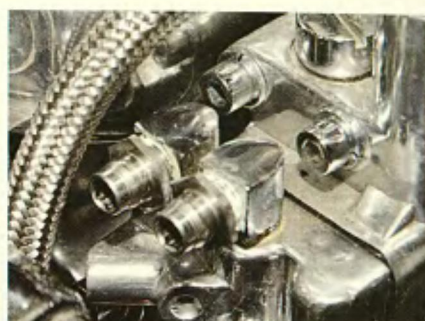
The male quick-connect fittings are screwed into the ports on the oil pump.
