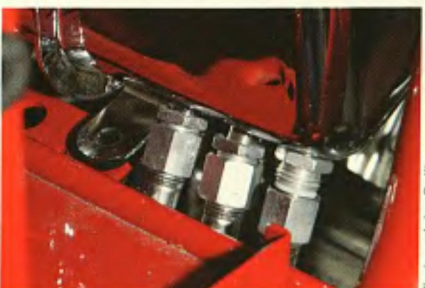
The working area under the oil tank is quite tight. But, by removing the starter and leaving the mounting bolts out of the oil tank, the new lines can be attached and tightened up.
